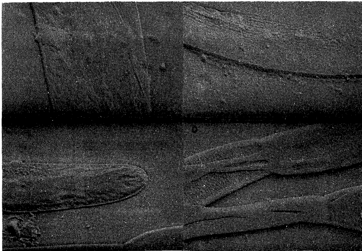
Figure 2: Scanning electron micrographs of resist images of foliar hairs of tomato (a) 60\text{mJ.cm}^{-2} soft X-ray fluence; (b) 40\text{mJ.cm}^{-2} soft X-ray fluence, and protonema of the moss Brachythecium (c), (d) 41\text{mJ.cm}^{-2} soft X-ray fluence.
