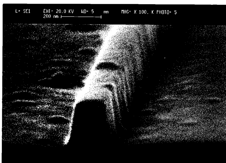
Figure 3. Patterned 200nm doped polysilicon gate electrode over 5nm thermal gate oxide.
