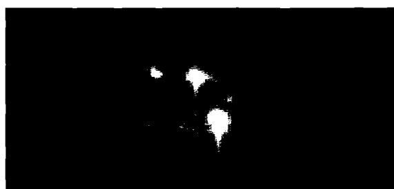
Figure 4. Far-field images of the second Stokes emission at 291 nm, showing the rays (upper image) and the bright spots (lower image), plus the on-axis ring pattern (visible in both).
