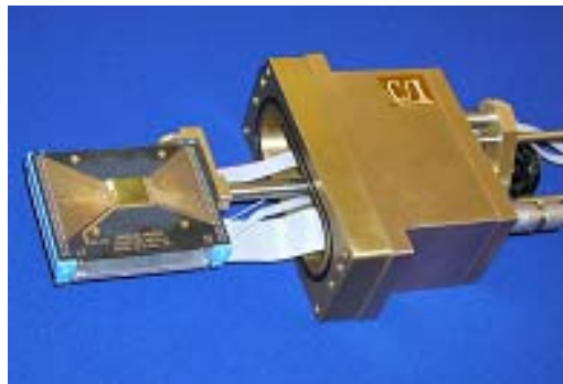
Figure 1. The CCLRC designed “Star Tracker” active pixel sensor.
