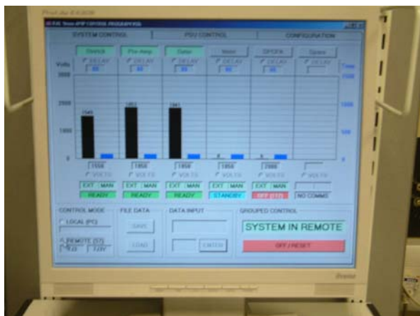
Figure 1. The computer interface used for the control of the 9mm pre-amplifiers.
